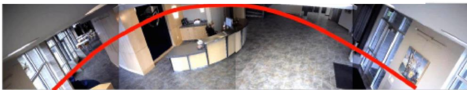
Figure 1E: Mounting height of 8ft and aimed only 30ft toward horizon
